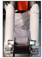
50. <u>Install the ski onto the spindle</u>: First make sure that the thick side of the ski rubber is toward the front. Adjust the bike so that the spindle bottom is slightly higher than the ski. Place the ski under the spindle and lift up on the front of the ski to pull it up into place. Note: It will be a tight fit between the ears of the ski bracket. Push the bolt through and install a lock washer on each side of the bolt. Torgue the nut to 50 ft.-lbs.
