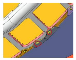
2.) From inside the tunnel install seven #7661637 rivets. The plates are directional, arrow towards front of snowmobile.
