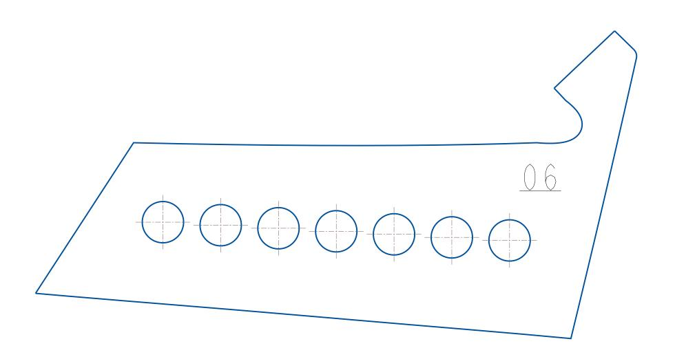
All Holes in Templates to be drilled to 5/8"
