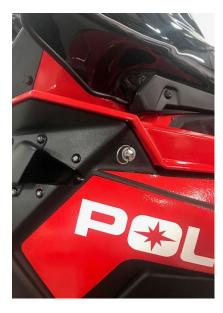
Left side panel in front of clutch. Locate straps and pegs relative to picture, making sure to have adequate tension on strap when installed. Make oblong hole that is  $1/4" \times 1"$  to insert strap thru, this is best done by using a step bit drilling 4- 1/4" holes and then blending in to create a 1" long oblong hole. Hole for stud/peg are 1" diameter, install 1"-20 1" flange head screw from back side of panel, install washer then t-nut add small amount of Blue Loctite then tighten.
