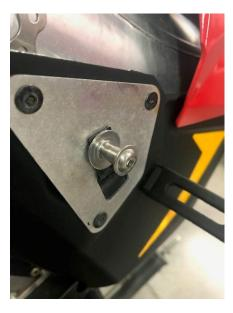
Lower rear both sides, install flange head screw with washer thru stock hole, install washer, Blue Loctite and t-nut then tighten securely. Locate strap relative to picture, drill 3/16" hole and rivet strap in place.
