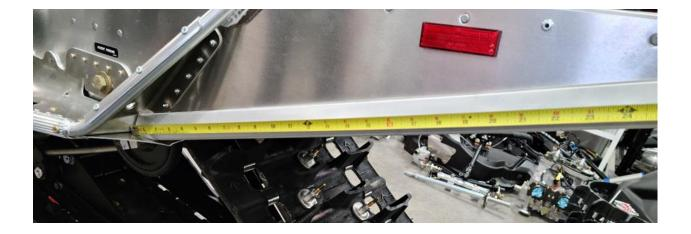
From each end of the rear bumper (see above picture for starting measuring point) measure up and make a mark at 21.125" and 22.125". Transfer the marks to the underside of the rear bumper. You will drill these holes in the rear bumper with a 3/16" Drill. The screws (7518280) will self-tap into the aluminum rear bumper.
