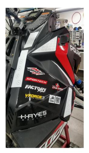
Holes drilled from templates (use a step bit to drill holes)
