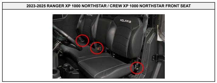
2. For multi passenger vehicles only, make sure the fasteners have been tightened by checking that the fasteners are tight and **DO NOT** move when turned by hand.
