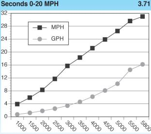
Test performed and verified by Yamaha Application Engineers.
