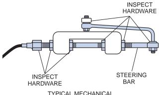
TYPICAL MECHANICAL OUTBOARD ENGINE STEERING LINK KC-0158-A
