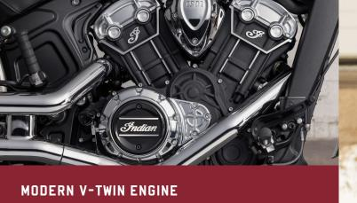
The liquid-cooled, 69 cubic inch V-twin makes a class leading 100 horsepower, delivering quick acceleration and plenty of power.
