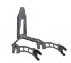
BOLT-ON PASSENGER SISSY BAR 2881127-650 Titanium Power Coat Paint. Requires Backrest Pad (2880827-01, -05) and Quick Release Accessory Mounting Spools (2881166), each sold separately. Fits 2015-2024 Scout & Scout Sixty.
