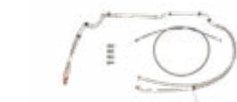
**Clutch Cable & Brake Line Kit**
