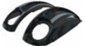
Injection-molded lids are precision-engineered and manufactured like stock lids. They host PowerBand™ Audio 6 1/2" Amplified Speakers and Speaker Bezels (each sold separately). These lids replace the Classic Saddlebag Lids. Color-matched with same premium finishes as stock lids. Install easily and fit perfectly. See page 115 for color options. Fits model year 2019 Chieftain® Classic & 2018-2019 Roadmaster®.
