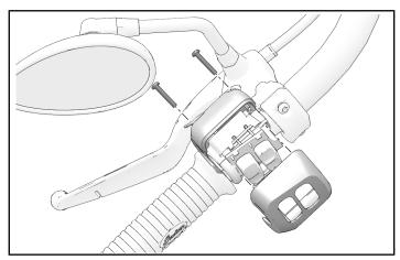
9. Align clutch handle assembly and beginning with top fastener, torque two fasteners to specification.
