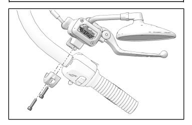
Twist throttle fully backward and forward to ensure throttle is properly seated and there is no dragging. If throttle is dragging, repeat installation.
