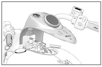
3. Remove and retain two switch fasteners. Remove and discard switch blank.
