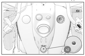
Carefully lift tank console from tank, reach under console and disconnect any connectors that may be installed. Carefully set tank console on protective surface
