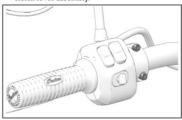
2. Slide and rotate clutch lever assembly to access outer cube fasteners. Use extra caution moving clutch lever assembly. Clutch lever wire is still connected to switch cube.
