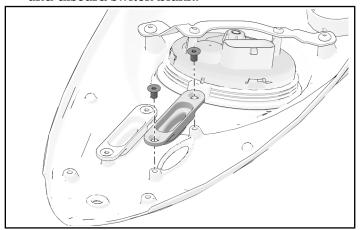
4. Install new switch and secure with two retained switch fasteners.
