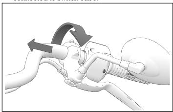
3. Remove two outer cube fasteners and remove two halves of cover.
