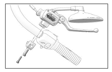
2. Remove two outer cube fasteners and remove two halves of cover.
