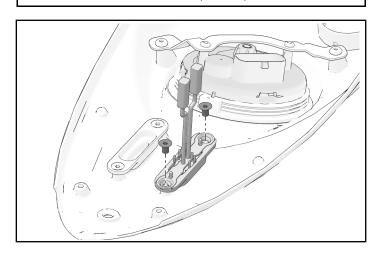
5. Plug heated grip switch connectors into corresponding connectors under console. Reconnect all other connectors under console.
