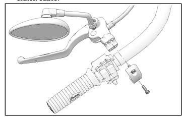
6. Remove two inner cube fasteners. Rotate switch side upward and remove entire assembly. Remaining connectors may stay connected as long as switch cube is supported.
