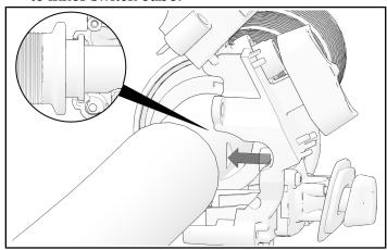
3. Close inner switch cube and reinstall two inner cube fasteners.
