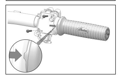
6. Loosely reinstall clutch lever assembly using two retained fasteners.
