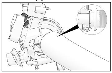
5. Quickly secure outer switch cube with two retained fasteners. Switch cube assembly notch should fit over tab on grip flange as shown with arrow. Rotate and adjust grip to fit properly.
