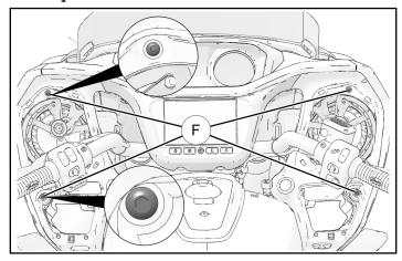
5. Loosely install three screws  $\widehat{\mathbb{E}}$  around headlight bezel as shown.
