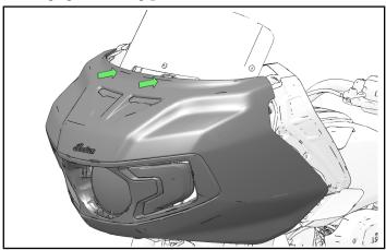
3. Loosely install one screw © into hole under edge of each side of fairing as shown. **DO NOT** torque fastener at this time.
