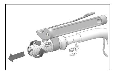
8. Use adhesive remover to clean adhesive residue or grip material from handlebar.
