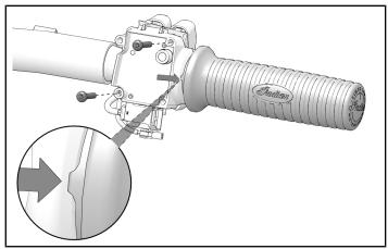
7. Connect heated grip connectors to switch cube assembly and wiring harness as shown.
