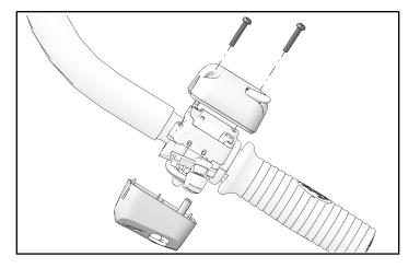
Reinstall brake lever assembly using two retained fasteners. Align handle and beginning with top fastener, torque two fasteners to specification.
