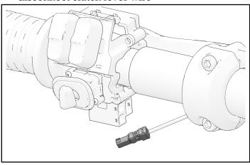
5. Remove two clutch lever assembly fasteners. Carefully let clutch lever assembly hang by clutch cable.
