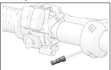
8. Reinstall left-hand switch cube cover using two retained fasteners. Ensure that all wiring is contained within switch cube. Ensure clutch wire is not pinched by two cube covers. Torque fasteners to specification.
