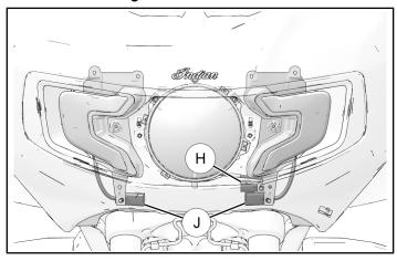
2. Press fairing into place and at top edge to engage locating pins.
