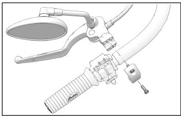
7. Connect clutch wire connector to switch cube assembly.
