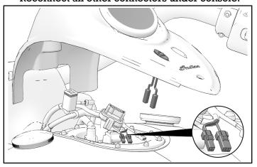
6. Reinstall tank console and secure with retained screws.
