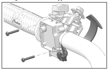
4. Slide and remove right-hand throttle tube/grip from handlebar.
