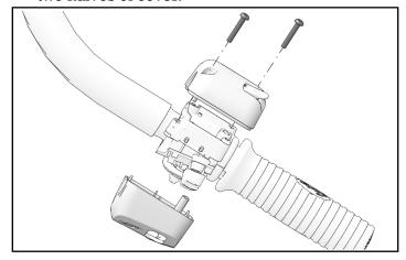
Remove two inner cube fasteners. Rotate switch side upward and remove entire assembly.
