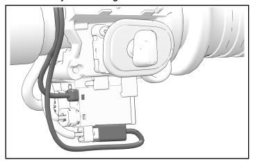
7. Reinstall right-hand switch cube cover using two retained screws. Ensure that all wiring is contained within switch cube. Torque fasteners to specification.
