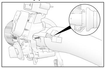
5. When inner switch cube is closed, heated grip wire should exit opening shown with arrow.
