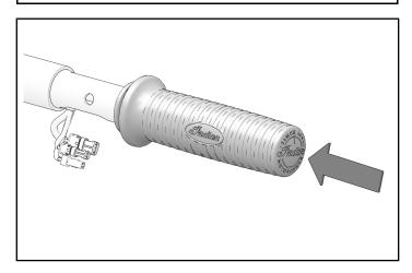
2. Orient inner switch cube so pin is inserted into handlebar. Ensure to line up slots in throttle tube to inner switch cube.
