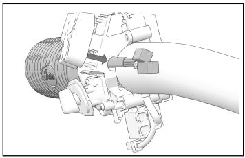
Quickly secure outer switch cube with two retained fasteners. Switch cube assembly notch should fit over tab on grip flange as shown with arrow. Rotate and adjust grip to fit properly.
