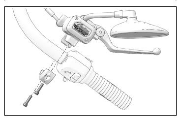
7. Twist throttle fully backward and forward to ensure throttle is properly seated and there is no dragging. If throttle is dragging, repeat installation.
