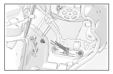
5. Join switch connectors to chassis harness wires, located on the side of storage compartment.
