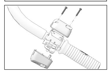
8. Reinstall brake lever assembly using two retained fasteners. Align handle and beginning with top fastener, torque two fasteners to specification.
