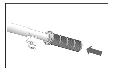
Quickly orient inner switch cube so pin is inserted into handlebar. Ensure to line up slots on left-hand grip to inner switch cube, as shown.
