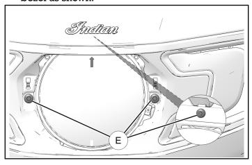
6. Torque all outer fairing screws to specification.
