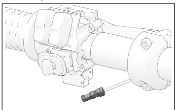
10. Reinstall left-hand switch cube cover using two retained fasteners. Ensure that all wiring is contained within switch cube. Ensure clutch wire is not pinched by two cube covers. Torque fasteners to specification.
