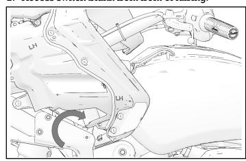
3. Remove and retain two switch fasteners. Remove and discard switch blank.
