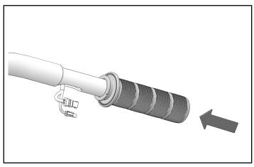
Quickly orient inner switch cube so pin is inserted into handlebar. Ensure to line up slots on left-hand grip to inner switch cube, as shown.
