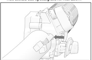
4. Close inner switch cube and reinstall two inner cube fasteners.
