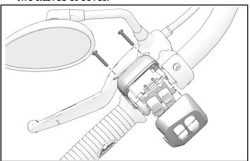
4. Use a small pick to release retaining tab and disconnect clutch lever wire
