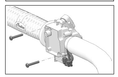
4. Twist throttle fully backward and forward to ensure throttle is properly seated and there is no dragging. If throttle is dragging, repeat previous two steps.
