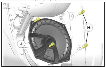
b. Connect electrical connectors to new speakers ① and set in place. Secure speakers using retained screws ④. Torque fasteners to specification.
