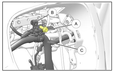
2. Unplug electrical connectors and remove and retain bolt ① and nut ⑥ from power supply module ⑥.
