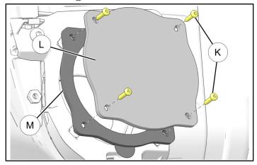
b. Connect electrical connectors to new speakers ① and set in place. Secure speakers using retained screws (k). Torque fasteners to specification.
