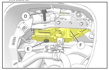
3. Remove power supply module (F) from RH fairing bracket.
