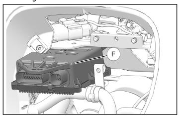
4. Install new power control module ② into RH fairing bracket in place of removed module. Ensure two tabs slide into bracket as shown. Plug in two connectors into module. Press connectors onto module until a "click" is heard.
