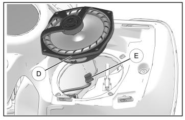
4. Connect electrical connector © to new speaker ①. Install speaker ① into fairing and secure with four retained screws ©. Torque screws © to specification.
