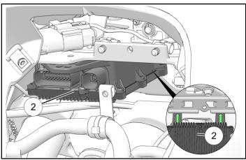
5. Secure new power supply module ② with new screw ③ and nut ④. Torque fastener to specification.
