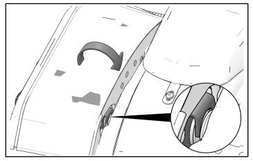
4. Open saddlebag and insert two screws ® through saddlebag and into spools. Handtighten two screws ®, to install saddlebag, before torquing to specification.
