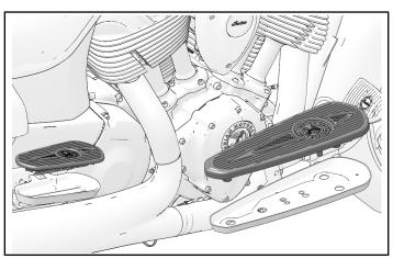
2. Ensure rubber protrusions are fully engaged with floorboard frame as shown.
