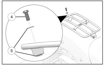
4. Torque rack mount screws to specification.
