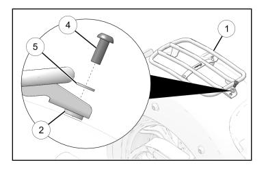
Lift rear of rack slightly and secure one washer
