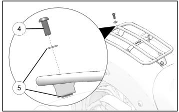
3. Torque rack mount screws to specification.
