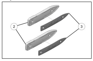
4. Put the exhaust tip tabs ② on the mufflers. Install the long screws ⑥ in the rear hole of each exhaust tip tab, and install the short screws ⑤ in the front hole of each exhaust tip tab. Torque screws to specification.
