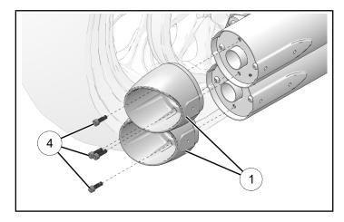
2. Remove the protective film from the outside of the exhaust badge ③ and adhesive film from the inside.
