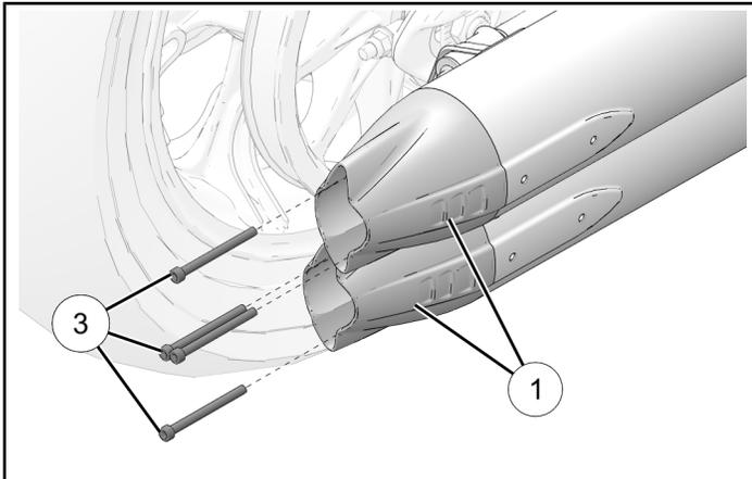
2. Remove the protective film from the outside of the exhaust badge ②.
