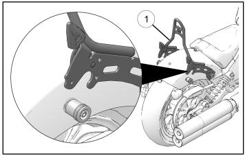
4. Close the backrest Lock & Ride® levers ® and install the retained safety screws ⓐ. Torque to specification.
