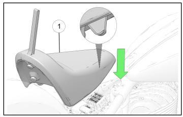
2. Install the washer and seat stud that were previously removed through the strap bracket on the seat ①. Torque the seat stud to specification.
