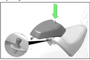
4. Insert the seat bracket screw 4 into the rear fender. Torque the screw to specification.
