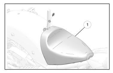
3. Insert the strap through the opening in the passenger seat. Engage the seat grommet to the seat stud by pressing down on the front of the passenger seat.
