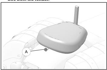
2. Remove the passenger seat ® by lifting up on the front edge of the seat to disengage the grommet from the seat stud.
