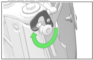
3. Standing in front of the vehicle, hold each side of the windshield and pull the windshield towards you to disengage the bracket mounts from the upper spools.
