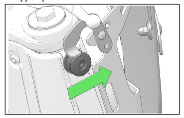
4. Lift the windshield straight up off the lower spools and off the vehicle.
