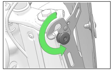
3. (Optional) Install one screw (9) through each latch and into the left-hand and right-hand bracket mount on each side of the vehicle. Torque the screws to specification.
