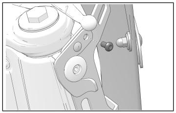
2. Locate and open the bracket mount latch on each side of the vehicle.
