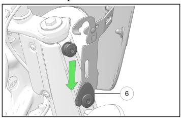
With the bracket mount latch open, push the windshield towards the rear of the vehicle to install into the upper spools. Rotate the latch around the upper spool on each side of the vehicle and close each latch.
