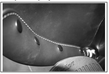
5. Make any adjustments to closeout so it is installed evenly on highway bar.
