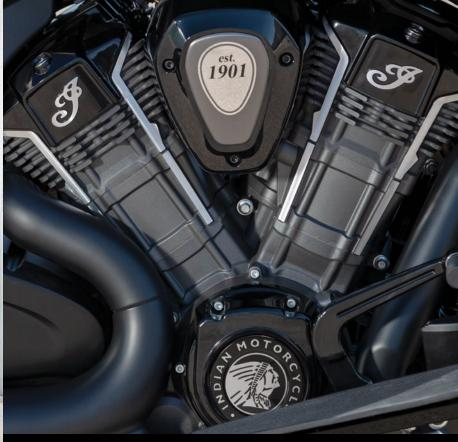
Our all-new liquid-cooled PowerPlus V-twin is the most powerful engine in its class. With overhead camshafts and four valves per cylinder delivering a blistering 122hp and 128 ft-lbs of torque, it redefines ultimate bagger performance.
