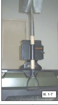
CAUTION: When loosening the clamping door turn knob, the door may swing open causing the saw to fall out. Make sure to hold onto saw when opening the saw clamping door.
