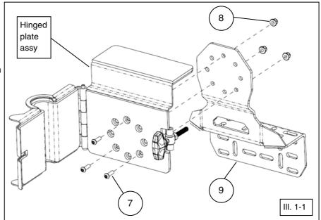
The hinged plate assembly can be set at 45 degree angle increments to the mount bracket to accommodate your UTV and Saw preferences. (See illustration 1-2).
