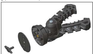
Insert the T-Bolt [Item 2] into the Lock & Ride MAX access hole and slide into the desired position along the rail. Assure that the track feature on the bottom of the Spacer Disc is positioned inside the opening of the rail.
