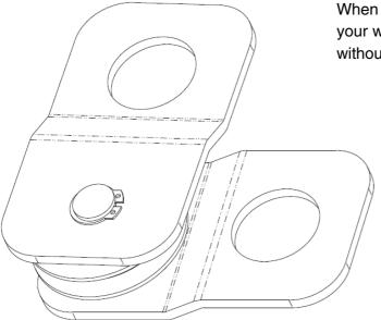
When properly used, the snatch block allows you to increase your winch's pulling power and change your pulling direction without damaging the cable.
