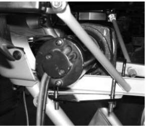
III. Insert the roller hawse mount plate (Item 2) between the winch mount plate (Item 1) and the winch. Set the winch onto the roller hawse mount plate, aligning the holes on the three components, using two M8 x 40mm bolts, two flatwashers and two nylock nuts. Note: The two spacers (Item 3), four 8x40 bolts (Item 8), two flatwashers (Item 6) and two lock nuts (Item 7) will not be used. Tighten at this time.
