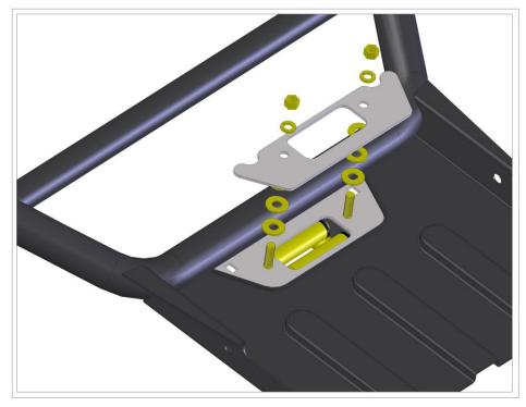
a) Step 1: Assemble the roller hawse, roller hawse plates, bolts, washers and lock nuts.
