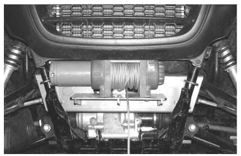
6) Place the front bumper on a work bench or the floor and install the roller hawse to the front bumper as shown in the image below.
