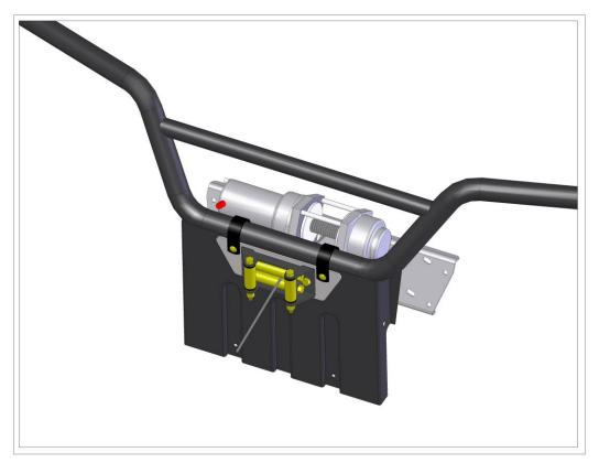
7) Feed the winch cable through the roller hawse rollers and reinstall the front bumper to the vehicle. (Depending on how large your cable end is, you may need to remove one of the long rollers and the two short rollers from the roller hawse and feed the winch cable through. Reinstall the rollers and be sure all rollers move freely.)
