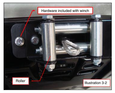
3. Using the hardware included with winch, fasten roller fairlead and the adapter plate to front bumper using bolts, washers and nuts. Tighten to specification. (See Illustration 3-2).
