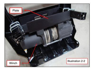
2. Position the winch in the front bumper assembly as shown. (See Illustration 2-2). *NOTE:* Winch is installed upside down and will function in this orientation.
