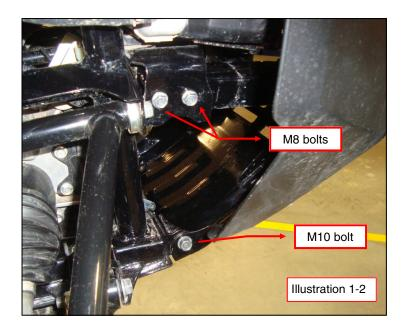
Position the winch mount plate, item 1, into the front bumper as far forward as it will go. Install square u-bolts, item 3, over frame tube and fasten with M8 flat washers, item 5, and M8 nuts, item 4, as shown. Torque to specification. (See Illustration 2-1).
