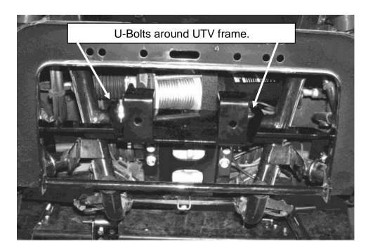
Install the winch to the winch mount plate and winch plate support and tighten all hardware at this time. Go to roller hawse instructions on page 7.
