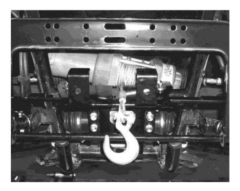
• Install the winch to the winch mount plate and winch plate support and tighten all hardware at this time. Go to Roller Hawse Instructions on page 7.
