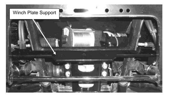
• Place the winch mount plate, Item #1 on top of the winch plate support and fasten the rear of the winch mount plate to the UTV with M8 x 35mm x 50mm U- bolts and nylock nuts. See picture on page 5. Do not tighten at this time.
