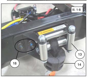
8MM FASTENER TORQUE: 17 ft. lbs. (23 Nm)
