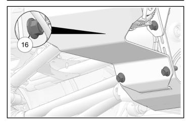
9. Torque winch assembly nuts  $(\)$  to specification.
