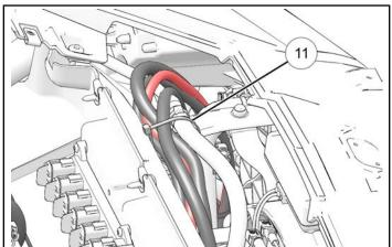
3. Continue routing harness through grommet in the lower dash wall and up towards the Pulse<sup>®</sup> Bar, use cable tie (1) to secure harness.
