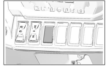
2. Pull switch connection through empty location and connect to switch. Connect green wire to pin one, red wire to pin 2, and black wire to pin 3 in rear of dash switch.
