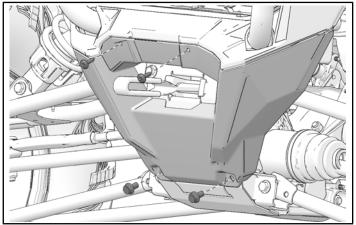
2. Remove two bolts. Remove front drive protection plate and tow strap.
