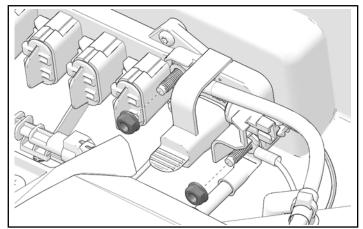
5. Attach positive and negative connections to Pulse<sup>®</sup> Bar using kept nuts.
