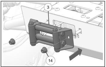
8. Torque winch assembly screws (6) until fully seated.
