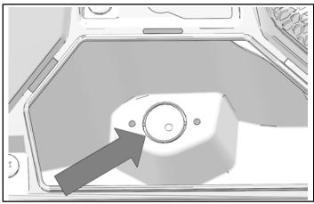
2. Route corded remote harness through the large hole and install dash socket using washers (5) and screws (3).
