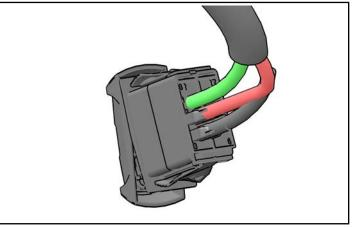
3. Install switch into empty location on dashboard, push switch until click is heard.
