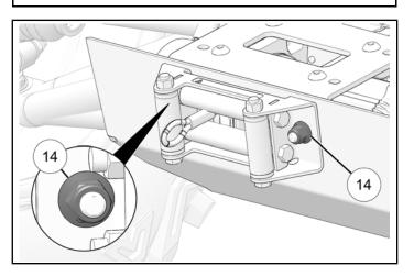
10. Install rubber bumper ④, hook ⑤ and strap ⑥ to winch rope.
