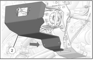
6. Loosely attach skid plate to vehicle frame with two screws (6).
