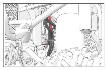
2. Continue routing harness up and over front left upper radiator support, use cable tie (1) to secure harness.
