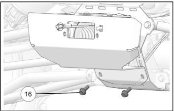
7. Install roller fairlead ③ onto skid plate and attach using two nuts ⑭.
