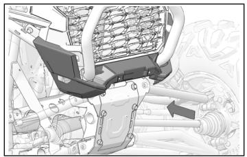
2. Install push-pin rivet to upper fascia.
