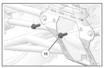
2. Install winch assembly ① onto vehicle frame by aligning upper key holes on winch assembly and lowering assembly onto screws <sup>(f)</sup>.
