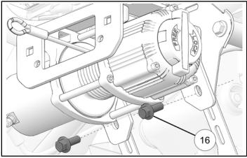
4. Loosely install two screws (1) to front of winch assembly.
