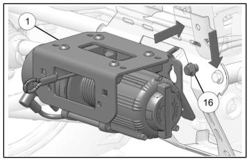
3. Attach winch assembly to vehicle frame with two screws (6).
