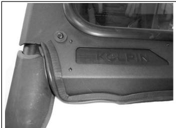
5. Put windshield on vehicle. Make sure bulb seal fits along top of dashboard.
