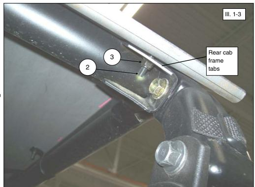
6. Continue to attach clamps (item #5) around the cab frame at each of the slotted hole locations. Fasten using M6 screws (item #2) and flat washers (item #3) through the top surface. Secure clamps into position from lower surface with M6 locknuts (item #4).
