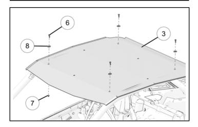
6. Attach the remaining two roof sides and the center of the rear and front roof with four screws (6) and washers (8), then place the four clamps (1), (2) around the cab frame tubes and fasten the screws with the nuts (7).
