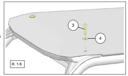
10. Install rear of roof using two of the shorter M6 screws (item #7) and flat washers (item #4) fitting thru two clamps (item #6) placed on rear cab frame crossmember tubing. Loosely fasten the rear clamp screws using two locknuts (item #5) as shown. (See illustration 1-8). Note: Do not tighten hardware at this step since adjustments may be required later.
