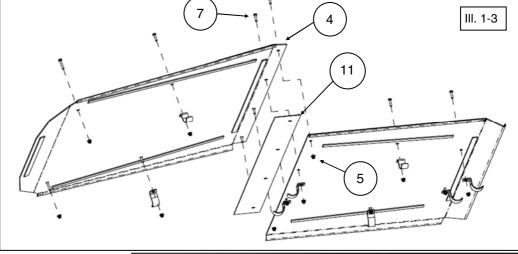
rubber seal (item #11) in between the two roof panels as shown. Do not tighten hardware at this step since adjustments may be required later.
