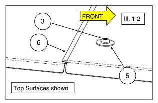
2. (Continued). Loosely secure with three M6 locknuts (item #4) on underside roof surface. (See illustrations 1-1 and 1-2). *Note, place rubber seal (item #6) in between the two roof panels as shown. Do not tighten hardware at this step since adjustments may be required later.*
