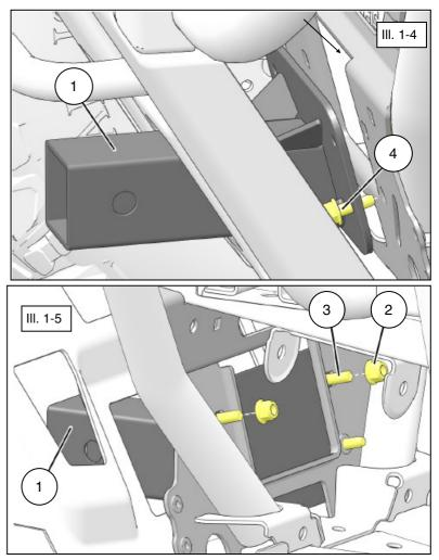
Newer Rangers with larger front gearcase: From rear side of vehicle frame, install SHCS screw (item #3) as shown. Fasten from front side using locknut (item #2). (See illustration 1-6).
