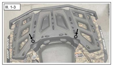
Attach the Left and Right Mounting Plates [Items 1 & 2] onto the OEM Rack as shown. Re-use the OEM M6 Locknuts underneath the OEM Rack. See III. 1-4.
