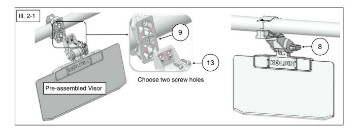
3. Tighten the screws to specified torque setting. **WARNING**: Do not over tighten hardware or damage can occur.
