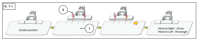
2. Tighten the screws to specified torque setting. WARNING: Do not over tighten hardware or damage can occur.
