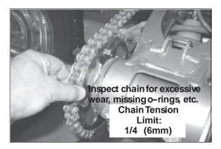
To check for wear, pull upward on the chain. Replace sprocket if chain movement exceeds 1/4 (.6 cm).
