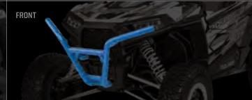
**1%" DIAMETER** STEEL TUBE CONSTRUCTION
