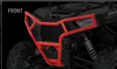
**1½" DIAMETER** STEEL TUBE CONSTRUCTION
