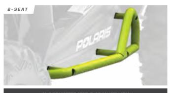
**1%" DIAMETER** STEEL TUBE CONSTRUCTION
