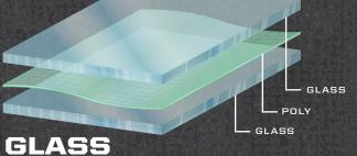
Superior OPTICAL CLARITY for a clear view. Laminated safety glass **PROTECTS FROM SCRATCHES** and provides automotive-level visibility.
