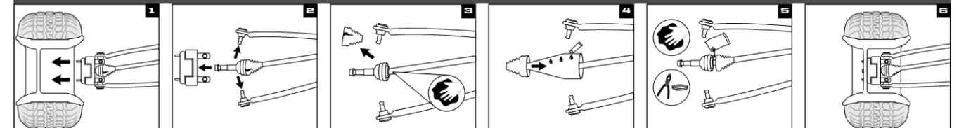
1. Remove wheel and axle nut.
