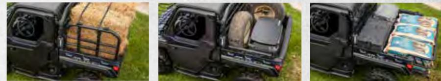
D'UN SIMPLE MOUVEMENT DE LEVIER, LES FIXATIONS LOCK & RIDE® UTILISENT LA PRESSION VERS L'EXTÉRIEUR POUR PRENDRE DE L'EXPANSION ET GARANTIR UNE FIXATION SÛRE.
