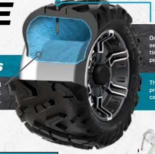
Once a leak occurs, the tire sealant rushes out of the tire and quickly creates a permanent solid plug.
