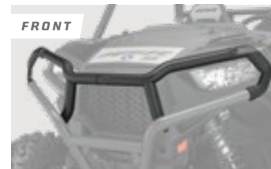
FRONT 1 1/4" DIAMETER STEEL TUBE CONSTRUCTION
