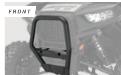
FRONT 1 1/2" x 2" STEEL OVAL CONSTRUCTION
