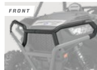
1 1/4" DIAMETER STEEL TUBE CONSTRUCTION
