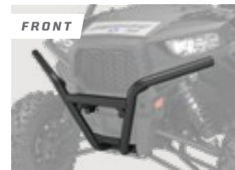
1 1/4" DIAMETER STEEL TUBE CONSTRUCTION
