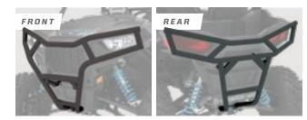
**1½" DIAMETER** STEEL TUBE CONSTRUCTION
