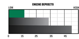
**Clean Engine Test** Lower Number = Less Deposits, Cleaner Engine Operates at Peak Performance. ASTM Test D6335
