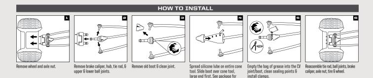
Refer to your service manual for further instructions and torque specifications. \*Designed for temporary CV boot repair. Purchase the OEM CV Boot for a permanent repair.
