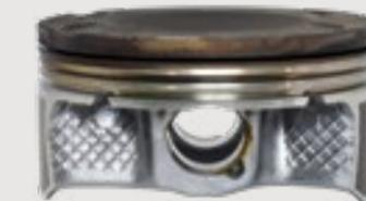
**PISTON RINGS & RING LANDS:** Extreme pressure to these parts require high lubricant film strength. Poor oxidative performance can lead to carbon and varnish buildup, which results in poor ring seal and fuel dilution of the oil. These can result in loss of power and accelerated engine wear.
