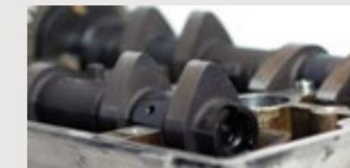
**CAMSHAFT:** Direct acting overhead camshafts are used on many Polaris engines. In this application the camshaft pushes directly on the valve, creating very high contact pressures compared to other camshaft configurations. These forces are so great that inferior oil can break down leading to increased wear and potential engine damage.
