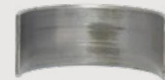
**ROD BEARINGS:** Engine bearings on an oil with low film strength and thinner viscosity can lead to premature wear or even engine failure.
