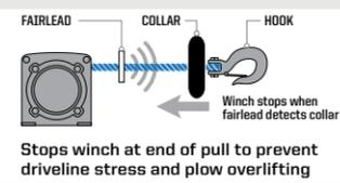
Stops winch at end of pull to prevent driveline stress and plow overlifting
